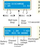
Set charge current on the left and the final voltage on the right. Range of the charge current is 0.1-1.0A; range of final voltage is 0.1-25.0V. Press START/ENTER key for more than 3 seconds to start the program.
