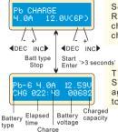
Set up the charge current on the left and nominal voltage on the right. Range of current is 0.1-5.0A, the voltage should match the battery being charged. Press START/ENTER key for more than 3 seconds to start charging.
