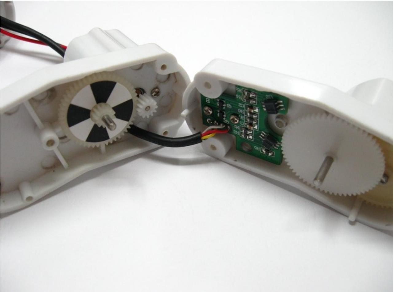
Each motor housing has two thick power wires that go directly to the motor. There are also 4 small wires with female headers.
