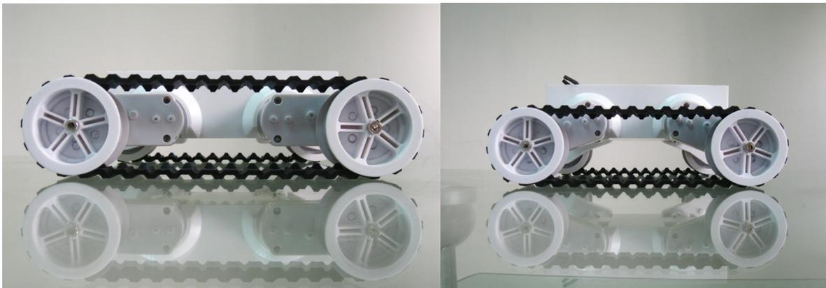
Each gearbox has an 87:1 ratio includes an optical quadrature encoder that gives 1000 pulses over 3 revolutions of the output shaft. The chassis can be upgraded to include four motors and encoders making it ideal for mecanum wheels.
