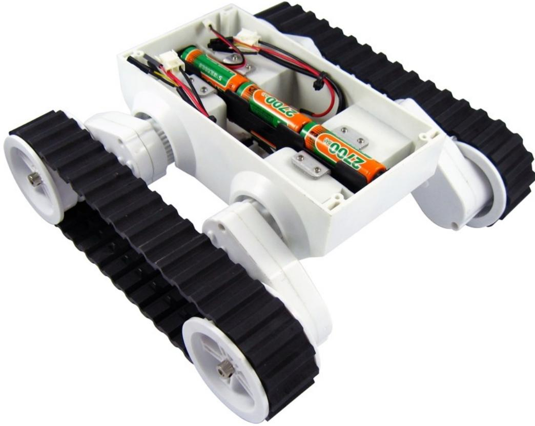
Rover 5 is a new breed of tracked robot chassis designed specifically for students and hobbyist. Unlike conventional tracked chassis's the clearance can be adjusted by rotating the gearboxes in 5-degree increments. "Stretchy" rubber treads maintain tension as the clearance is raised.
