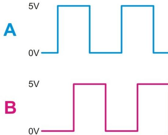
If you only wish to monitor the speed of rotation then you can use either output and simply measure the frequency. The reason for having two outputs is that you can also determine the direction of shaft rotation by looking at the pattern of binary numbers generated by the two outputs. Depending on the direction of rotation you will get either:
