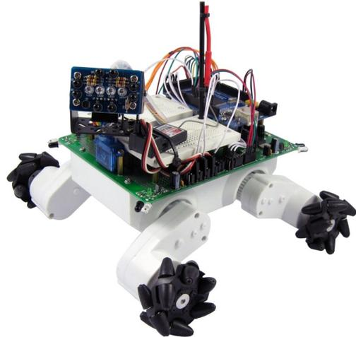
Inside of the chassis are 4 noise suppression coils at the bottom and a battery holder that accepts 6x AA batteries. It is recommended to use NiMh batteries as they last longer and have a higher current output than Alkaline batteries.
