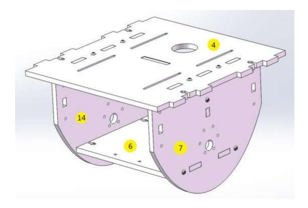
**6.** Fix both No.14 and the No.5 part into the notch of the No.4 part. And fix the screws on.
