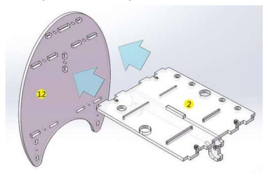
2. Then fix the No.2 part into the notch of the No.12 part.
