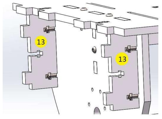
7. Fix the No.13 part into the notch of the notch of the No.14 part and
