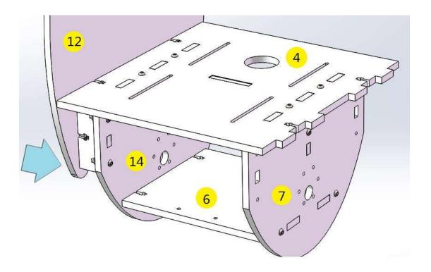
**8.** Fix all of the part which finished by the last step into the No.12 part.
