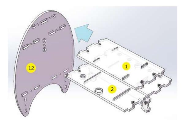
**3.** Fix the No.1 part into the notch of No.12
