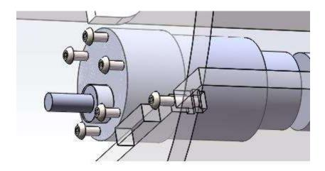
**10.** Fix the motors on the robot.
