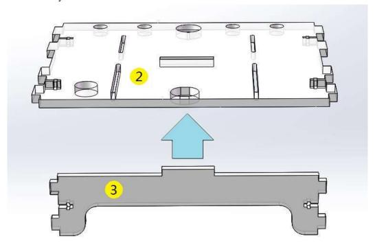
1. Fix the No.3 part into the notch of the No.2 part
