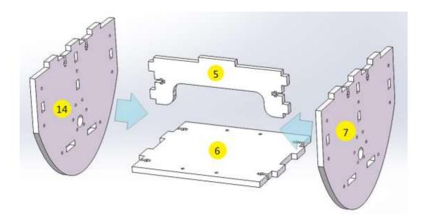
5. Fix each side of both No.5 part and No.6 part to the notch of both No.14 part and No.7 part
